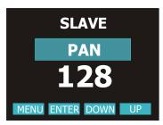
signal from the MASTER unit. By setting all the SLAVE units connected to the MASTER, to DMX address 1, them will be synchronized with the Master unit following the chase selected on it, but running their own Pan&Tilt and Zoom position.
