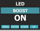
BOOST With BOOST active, the LED's current is set to 500 mA (30% more gain) Default = Enabled
